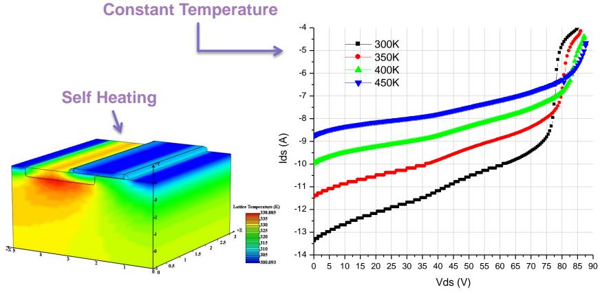
Vg=12V Vd=55V Self-heating with thermal conductance of 0.1 W/mK
