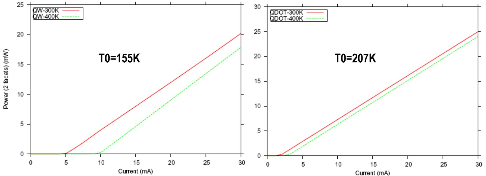
**Comparison of lasing behavior at 300 and 400 K. All structures are forced to lase at 1.17 microns and temperature dependences in bandgap, optical gain, carrier concentration, and radiative recombination have been taken into account. All other quantities are assumed to be temperature independent for simplicity**
