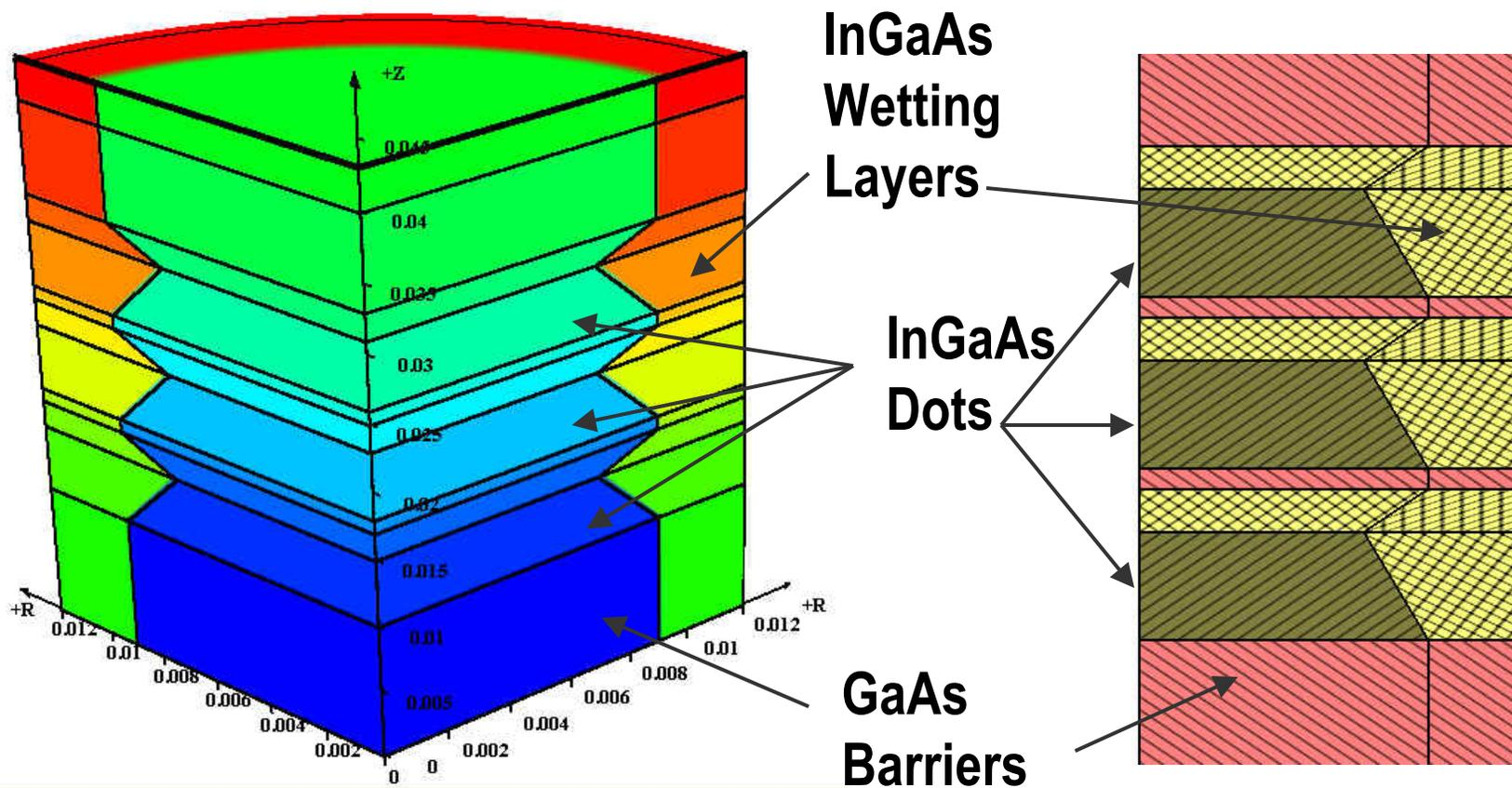
Remark: It is a simplified structure. Real structure Of QDOT may have composition grading from InGaAs To InAs at the center of the dot.
