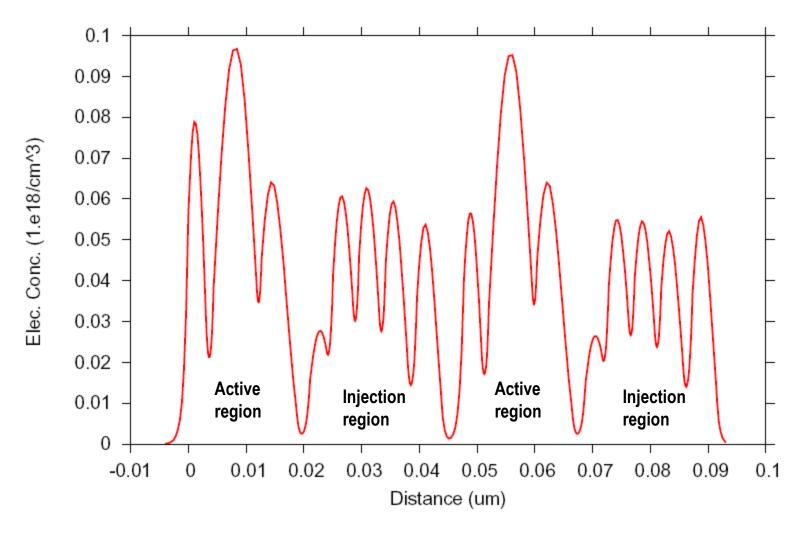
Electron distribution based on subband population calculated by microscopic rate equations
