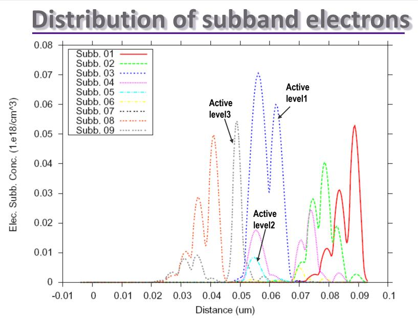
First 9 levels are plotted with the first three levels in active region labeled
